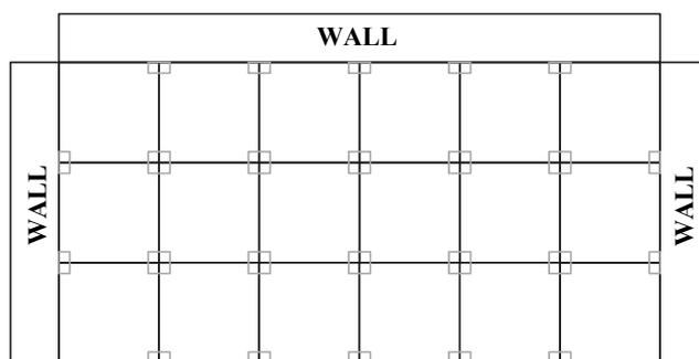
**Install tabs to the back of each tile so that one quarter of each tab contacts an individual tile. Use half tabs at walls.**
